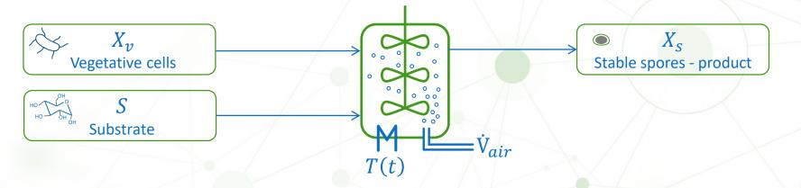
Process optimization: Find the optimal temperature trajectory to minimize the batch time
